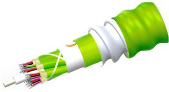
Fiber indoor cable, LazrSPEED® Riser/LSZH rated Distribution, interlocking aluminum armored, Multimode OM5, 12 fiber single-unit, Feet jacket marking, Lime-green jacket color
