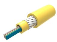
Fiber Indoor Cable, Plenum All-Dielectric Central Tube Ribbon, 12-fiber, Singlemode G.652.D and G.657.Al, Feet jacket marking, Yellow jacket color
