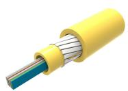
Fiber Indoor Cable, Plenum All-Dielectric Central Tube Ribbon, 60-fiber, Singlemode G.652.D and G.657.Al, Feet jacket marking, Yellow jacket color
