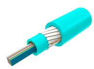
Fiber Indoor Cable, Plenum All-Dielectric Central Tube Ribbon, 48-fiber, Multimode OM3 bend insensitive, Feet jacket marking, Aqua jacket color
