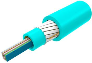
Fiber Indoor Cable, Plenum All-Dielectric Central Tube Ribbon, 96-fiber, Multimode OM4 bend insensitive, Feet jacket marking, Aqua jacket color
