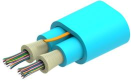
Fiber indoor cable, LazrSPEED® Plenum for MPO Trunks, 48 fiber with 24 fiber subunits, Multimode OM5, Feet jacket marking, Lime green jacket color
