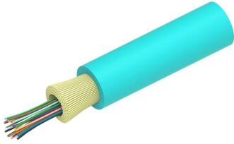
Fiber indoor cable, LazrSPEED® Low Smoke Zero Halogen Riser Light Duty for MPO Patchcords, 24 fiber, Multimode OM5, Gel-free, Feet jacket marking, Lime green jacket color, Dca Flame rating
