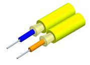
Fiber indoor cable, 2.0 mm diameter, Riser rated, Zipcord 2-fiber, Singlemode G.657.B3, Feet jacket marking, Yellow jacket color
