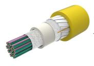
Fiber indoor/outdoor cable, All-Dielectric, LSZH, Riser-Rated, Gel-Free, Central Tube Rollable Ribbon, 144 fiber, Singlemode G.657.A2/B2, Feet jacket marking, Yellow jacket color, Cca flame rating
