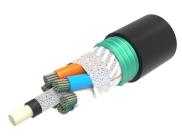
Fiber OSP cable, Outdoor Steel Armored, Gel-Free, Stranded Loose Tube Rollable Ribbon, 1728 fiber, Singlemode G.652.D and G.657.A1, Feet jacket marking, Black jacket color, Build America Buy America (BABA)
