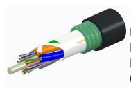
Fiber indoor/outdoor cable, TeraSPEED®, Single Jacket/Single Armor, Low Smoke Zero Halogen (LSZH), 96 fiber, Singlemode G.657.A2, Gel Filled, Stranded Loose Tube, Black jacket color, Meters jacket marking, Cca flame rating
