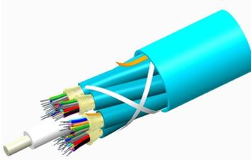
Fiber indoor cable, LazrSPEED® Plenum Distribution, 48-Fiber Multi-Unit with 12-Fiber Subunits, Multimode OM4, Gel-free, Feet jacket marking, Violet jacket color
