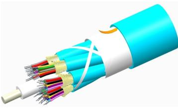
Fiber indoor cable, LazrSPEED® Low Smoke Zero Halogen Riser Distribution, 72 fiber multi-unit with 12 fiber subunits, Gel-free, Multimode OM3, Feet jacket marking, Aqua jacket color
