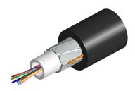
Fiber Indoor/Outdoor Drop Cable, LazrSPEED®, Low Smoke Zero Halogen, 24 fiber, Single Jacket All-Dielectric Arid-Core, Gel-filled, Multimode OM3, Feet jacket marking, Black jacket color, Dca flame rating
