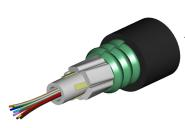
Fiber drop cable, TeraSPEED® Single Jacket Single Armor Arid-Core, 2-fiber, Singlemode G.652.D and G.657.A1, gel-filled, Feet jacket marking, Black jacket color
