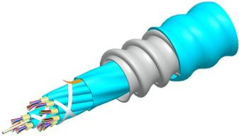
Fiber indoor cable, LazrSPEED® Riser/LSZH rated, MPO Trunk, interlocking aluminum armored, Multimode OM4, 12 fiber, Gel-free, Feet jacket marking, Aqua jacket color, B2ca flame rating
