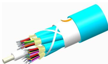
Fiber indoor cable, TeraSPEED® Low Smoke Zero Halogen Riser Distribution, 48 fiber multi-unit with 12 fiber subunits, Gel-free, Singlemode + Multimode OM3, Feet jacket marking, Aqua jacket color, Cca flame rating
