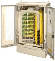
FDH 3000 Small Fiber Distribution Cabinet, 144F, SC/APC, (2) 16-splitter modules, dielectric loose tube, 100 ft, 24F
