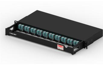
1RU patch panel which interfaces with MPO-8 ports including QSFP to easily break them out into LC connections. The MPO and shuttered LC ports are both front facing for easy mapping and patching. 10 MPO-8 and 40 duplex LC ports, OM4, Enhanced Method B
