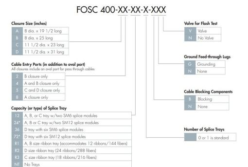
\*Note: SMOUV (1120-01-US) splice protection sleeves should be used with SM12 splice modules.
