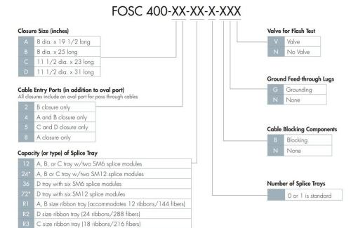
\*Note: SMOUV (1120-01-US) splice protection sleeves should be used with SM12 splice modules.
