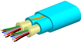
Fiber indoor cable, LazrSPEED® Plenum MPO Trunk, 24 fiber with 12 fiber subunits, Multimode OM3, Feet jacket marking, Red jacket color
