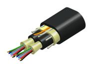
Fiber Indoor/Outdoor cable, TeraSPEED® Low Smoke Zero Halogen Riser MPO Trunk, 24 fiber with 12 fiber subunits, Gel-free, Singlemode G. 652.D and G.657.A1, Feet jacket marking, Black jacket color, Dca flame rating
