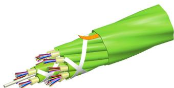
Fiber indoor cable, LazrSPEED® Plenum MPO Trunk, 72 fiber multi-unit with 12 fiber subunits, Multimode OM5, Gel-free, Feet jacket marking, Lime green jacket color
