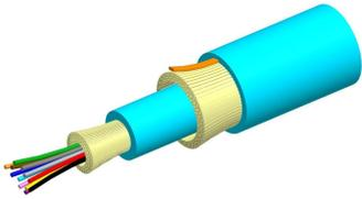
Fiber indoor cable, LazrSPEED® Plenum for MPO Trunks, 12 fiber, Multimode OM4, Feet jacket marking, Aqua jacket color
