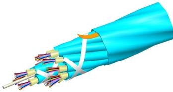
Fiber indoor cable, LazrSPEED® Plenum MPO Trunk, 48 fiber multi-unit with 12 fiber subunits, Multimode OM4, Gel-free, Feet jacket marking, Aqua jacket color
