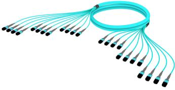
Ultra Low Loss (ULL) OM4, MPO8 QSFP Unpinned to MPO8 QSFP Pinned, Fiber Trunk Cable Assembly, 96-Fiber, Plenum
