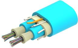
Fiber indoor cable, LazrSPEED® Low Smoke Zero Halogen Riser MPO Trunk, 48 fiber with 24-fiber, 3.0 mm subunits, Multimode OM4, Feet jacket marking, Aqua jacket color, B2ca flame rating
