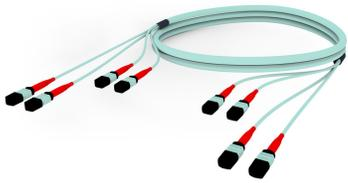
Ultra Low Loss (ULL) OM4 MPO24 (Pinned) to MPO24 (Pinned), Fiber Trunk Cable Assembly, 96-Fiber, Low Smoke Zero Halogen (LSZH)
