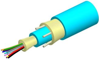
Fiber indoor cable, LazrSPEED® Low Smoke Zero Halogen Riser MPO Trunk with 2.0mm Subunits, 12 fiber, Multimode OM4, Gel-free, Feet jacket marking, Aqua jacket color, Dca flame rating
