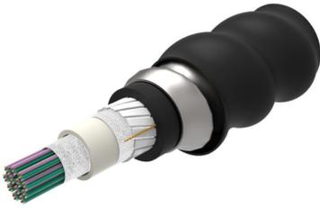
Fiber indoor/outdoor cable, Interlocking Armored, LSZH Riser-Rated, Gel-Free, Central Tube Rollable Ribbon, 864 fiber, Singlemode G.657.A2/B2, Feet jacket marking, Black jacket color, B2ca flame rating
