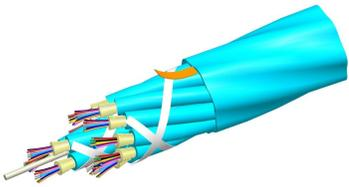
Fiber indoor cable, Plenum MPO Trunk, 36 fiber multi-unit with 12 fiber subunits, Singlemode G.657.A2/B2, Feet jacket marking, Yellow jacket color
