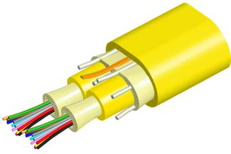
Fiber indoor cable, Low Smoke Zero Halogen Riser MPO Trunk, 24 fiber with 12 fiber subunits, Singlemode G.657.A2/B2, Gel-free, Feet jacket marking, Yellow jacket color, Dca Flame rating
