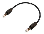
D-CLASS HELIAX® 1/2" Superflexible SureFlex® Jumper with interface types 4.3-10 Male and 4.3-10 Male with HELIAX® SureGuard weatherproofing, 15.5m
