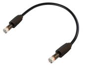
HELIAX 1/2" Superflexible SureFlex® Jumper with interface types 7-16 DIN Male and 7-16 DIN Male with HELIAX® SureGuard weatherproofing, 3.5 m
