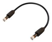
HELIAX® 1/2" Superflexible Fire retardant SureFlex® Jumper with interface types 4.3-10 Male and 7-16 DIN Male with HELIAX® SureGuard weatherproofing, 1.5m, with black non-halogenated fire retardant polyolefin jacket B2ca-S1a-d1-a1
