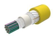
Fiber indoor/outdoor cable, All-Dielectric, LSZH/Riser-Rated, Gel-Free, Central Tube Rollable Ribbon, 576 fiber, Singlemode G.657.A2, Feet jacket marking, Yellow jacket color, Cca flame rating
