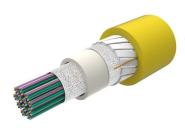
Fiber indoor/outdoor cable, All-Dielectric, LSZH/Riser-Rated, Gel-Free, Central Tube Rollable Ribbon, 576 fiber, Singlemode G.657.A2, Feet jacket marking, Yellow jacket color, Cca flame rating
