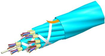
Fiber indoor cable, Low Smoke Zero Halogen Riser MPO Trunk, 96 fiber multi-unit with 12 fiber 2.0mm subunits, Gel-free, Singlemode G.657.A2 /B2, Feet jacket marking, Yellow jacket color, Dca flame rating
