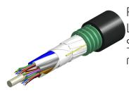
Fiber indoor/outdoor cable, LazrSPEED®, Single Jacket/Single Armor, Low Smoke Zero Halogen (LSZH), 144 fiber, Multimode OM4, Gel Filled, Stranded Loose Tube, Black jacket color, Meters jacket marking, Cca flame rating
