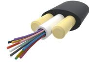
Fiber outdoor drop cable, LightScope® ZWP Self-Supporting All-Dielectric, Singlemode G.652.D and G.657.A1, 8 fiber Arid Core construction, Gel-filled, central loose tube, no ripcords, Feet jacket marking, Black jacket color
