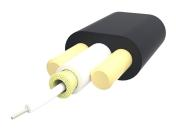
Fiber Universal Service Drop Cable, dielectric, with 900um Buffer, 1-fiber, Singlemode G.657.A2/B2,Gel-free, Feet jacket marking, Black jacket color
