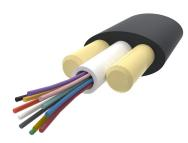
Fiber outdoor drop cable, LightScope® ZWP Self-Supporting All-Dielectric, Singlemode G.652.D and G.657.Al, 1–fiber Arid Core construction, Gel-filled, central loose tube, no ripcords, Feet jacket marking, Black jacket color
