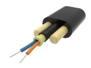
Fiber outdoor drop cable, Self-Supporting All-Dielectric, 2 fiber construction, Interconnect, Singlemode G.657.A2/B2, Gel-free, Feet jacket marking, Black jacket color
