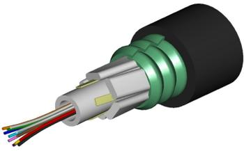
Fiber drop cable, LightScope® ZWP Single Jacket Single Armor Outdoor Drop Cable, 6 fiber Arid Core construction, central loose tube, Gel-filled, Singlemode G.652.D and G.657.A1, Feet jacket marking, Black jacket color
