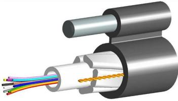
Fiber drop cable, TeraSPEED® Self-Support Figure-8 Single Jacket Non-Armor Arid-Core, central loose tube, 6 fiber, Singlemode, G.652.D and G.657.A1, Gel-filled, Feet jacket marking, black jacket color
