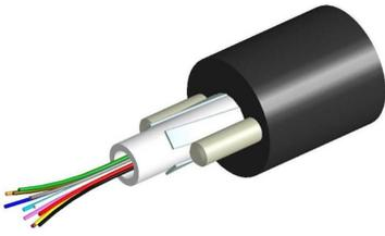
Fiber outdoor drop cable, LightScope® ZWP All-Dielectric, 4 fiber Arid Core construction, central loose tube, Singlemode G.652.D and G.657.A1, Gel-filled, Feet jacket marking, Black jacket color
