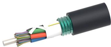
Fiber OSP cable, LightScope® ZWP Single Jacket/Single Armor, Gel-Free, Stranded Loose Tube, 24 fibers, Singlemode G.652.D and G.657.A1, Feet jacket marking, Black jacket color
