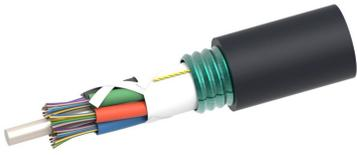
Fiber OSP cable, LightScope® ZWP Single Jacket/Single Armor, 60 fibers, Gel-Free, Stranded Loose Tube, Singlemode G.652.D and G.657.A1, Feet jacket marking, Black jacket color
