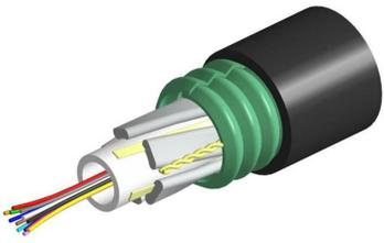
Fiber drop cable, LightScope® ZWP Single Jacket Single Armor Outdoor Drop Cable, 12 fiber Arid Core construction, central loose tube, Gel-filled, Singlemode G.652.D and G.657.A1, Feet jacket marking, Black jacket color
